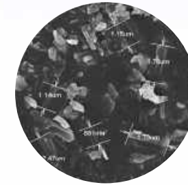
Particle size of the drug coating under 8.8mmx10.0k electron microscope
